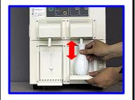
Use the server sake bottle to ajust the holder. (Be sure the nozzle reach inside the server bottle).
