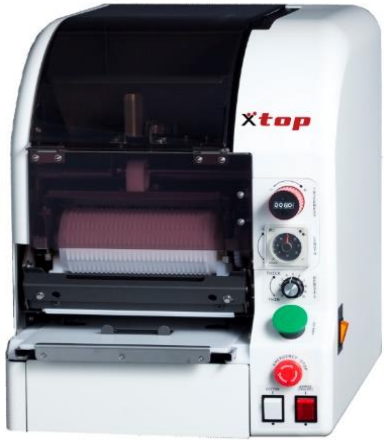
Sushi Rice Sheet Robot TSM-900RS
